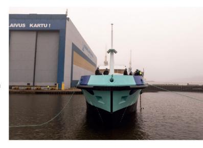
Workboats, Estonia, at a reported cost of €12 million. Designed for a three-person crew, the 42m x 10m newbuild has the capacity to store 400m³ of liquid waste, and its features include a range of special tanks and treatment systems, including a rainwater treatment plant, to filter the water before it is moved to treatment facilities on shore.
