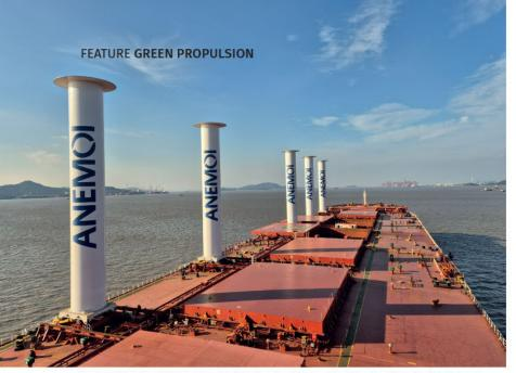
Sohar Max is claimed to be the largest vessel yet to be fitted with WAPS
