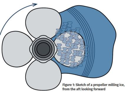
The frequency for the propeller ice-milling loads was simply defined as the blade order frequency.
