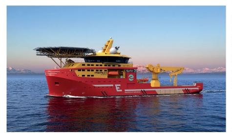
The forthcoming CSV, due in 2027, will run on batteries and a choice of methanol or MGO
