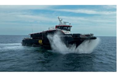
As you'd expect, it does demand a lot of power: there are four meaty, 1,440kW MTU 16V2000 M72 engines, two in each leg. The extra space at the rear is necessary to accommodate the four S50-3/CA Kongsberg waterjets.
