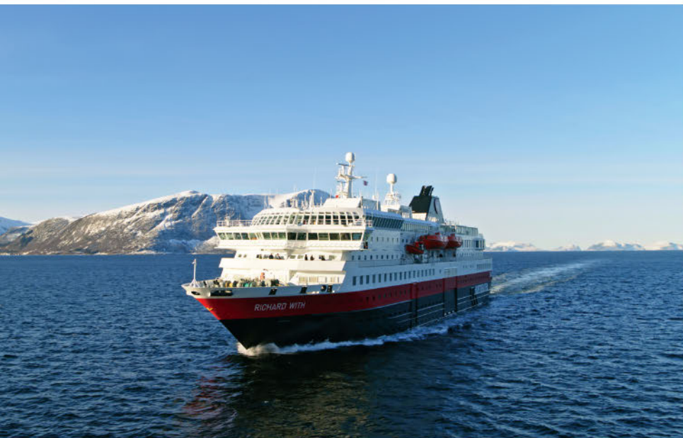
HURTIGRUTEN'S MS RICHARD WITH HAS BEEN CONVERTED TO HYBRID OPERATIONS. SOURCE: HURTIGRUTEN
