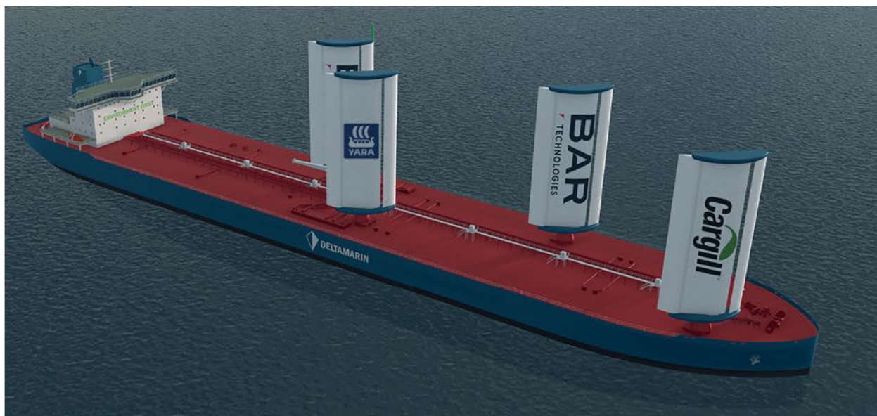
BARA AND YARA ARE MARKETING THE WINDWING SOLID SAIL SYSTEM. SOURCE: YARA MARINE
