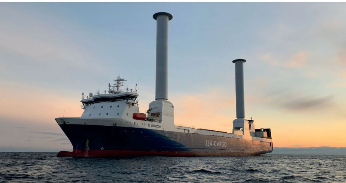
TILTING FLETTNER ROTORS ON SC CONNECTOR SHOW EVOLUTION OF MODERN WIND TECHNOLOGY
