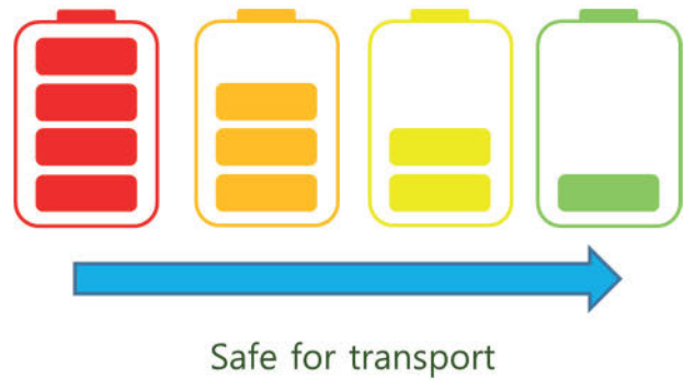
FIG 2: SAFE TRANSPORTATION IS INTRINSICALLY LINKED TO THE LITHIUM-ION BATTERY'S STATE OF CHARGE
