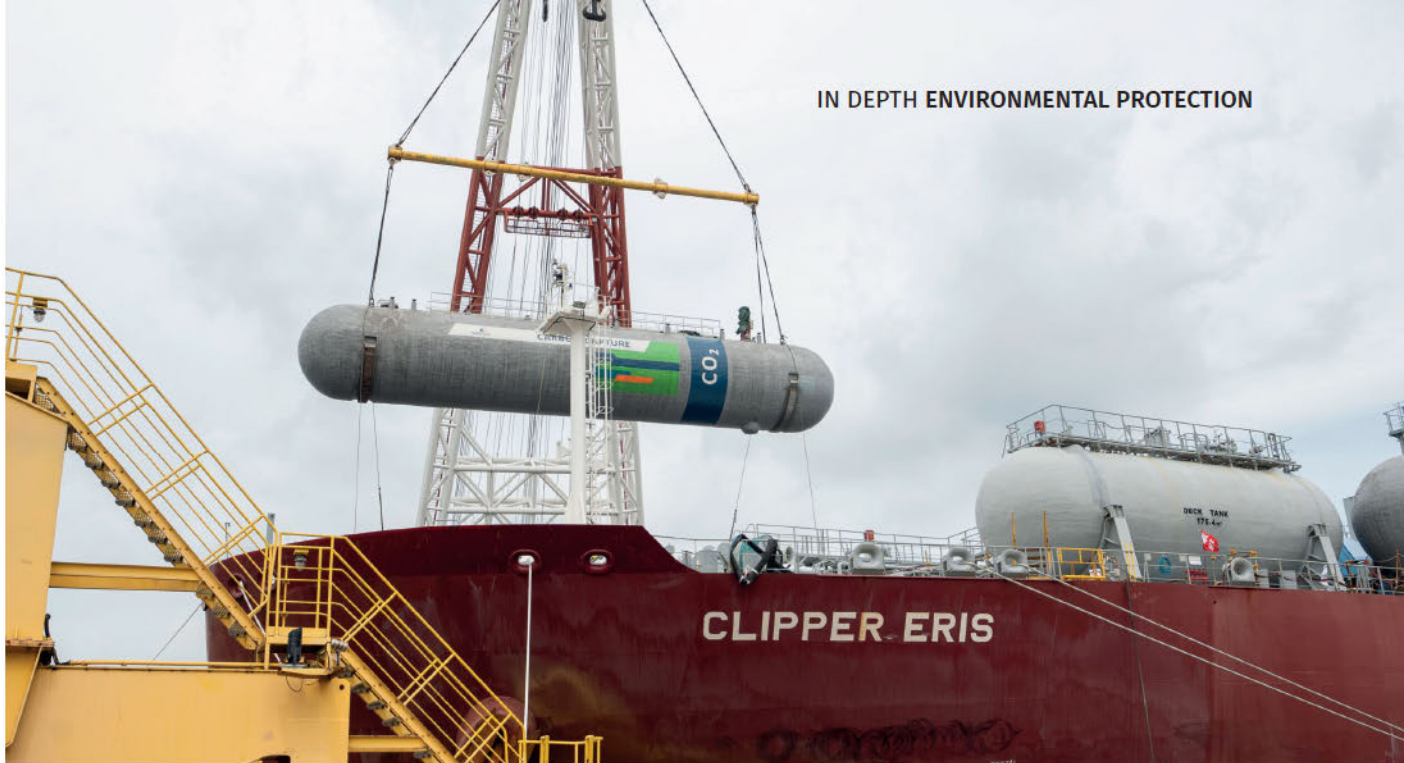
Carbon capture tanks being loaded onto Clipper Eris during its retrofit in Singapore earlier this year
