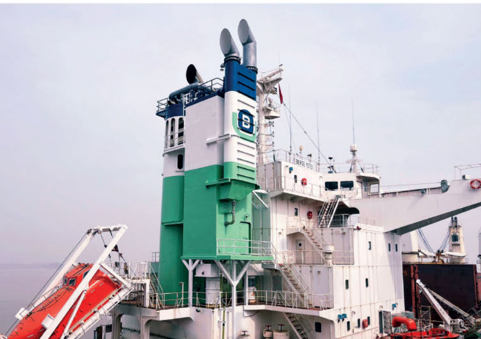
Berge Bulk recently retrofitted Berge Yotei with a Value Marine exhaust gas filter and carbon capture system
