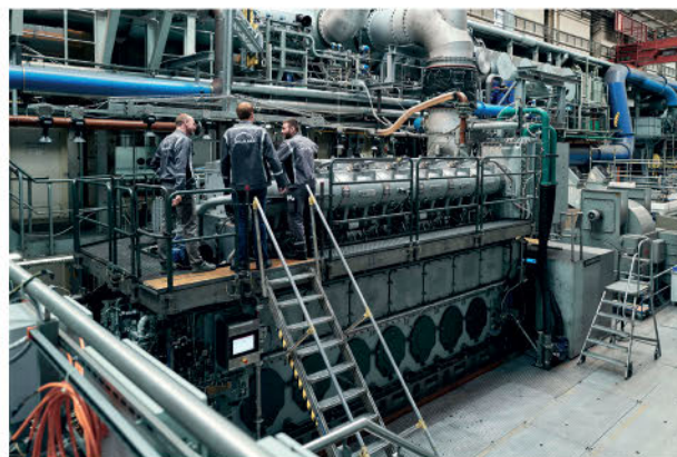
FROM 2025 OWNERS WILL BE ABLE TO HAVE CONVENTIONAL MAN 48/60 ENGINES CONVERTED TO NEW MAN 51/60R-DF-M ENGINES, BOTH WITH OR WITHOUT A COMMON-RAIL SYSTEM
