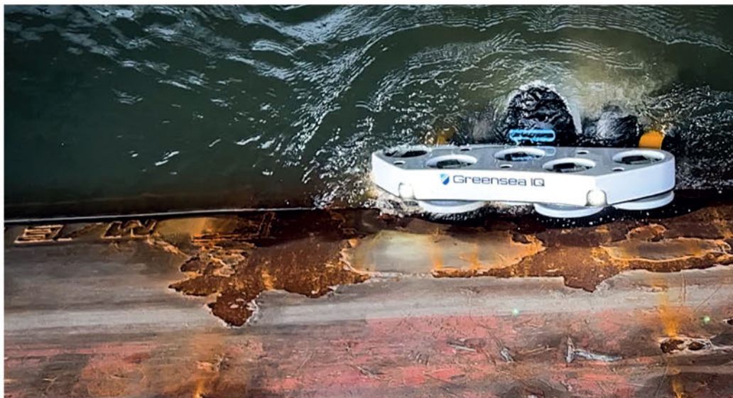
THE GREENSEA IQ EVERCLEAN HULL CLEANING ROBOT IN ACTION
