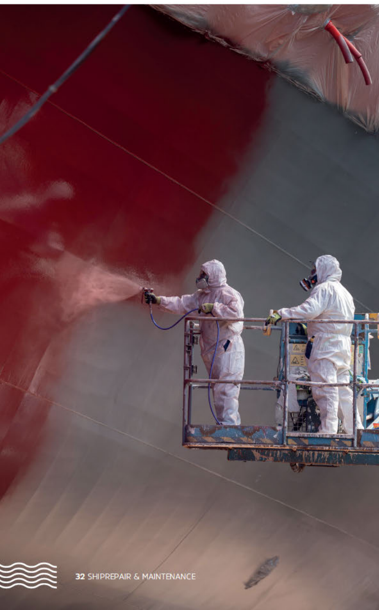
SHIPYARD STAFF APPLYING GIT'S GRAPHENE-BASED COATINGS ON A VESSEL HULL DURING DRYDOCKING
