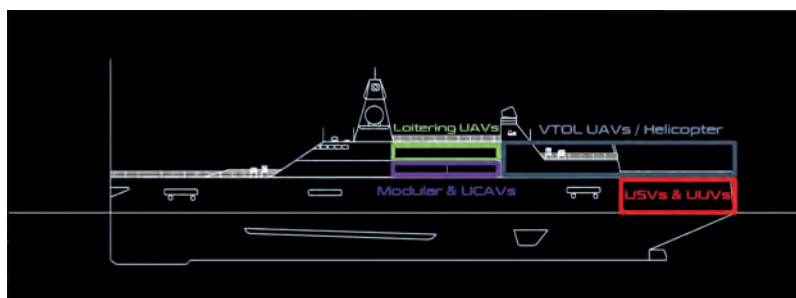
THE DRONE SHIP CONCEPT MERGES CHARACTERISTICS OF SURFACE COMBATANTS SUCH AS FRIGATES, DESTROYERS AND CRUISERS AND AIRCRAFT CARRIERS
