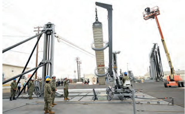
TRAM WILL ENABLE US NAVY SURFACE COMBATANTS TO RELOAD MISSILE CANISTERS INTO MK 41 VLS WHILST AT SEA
