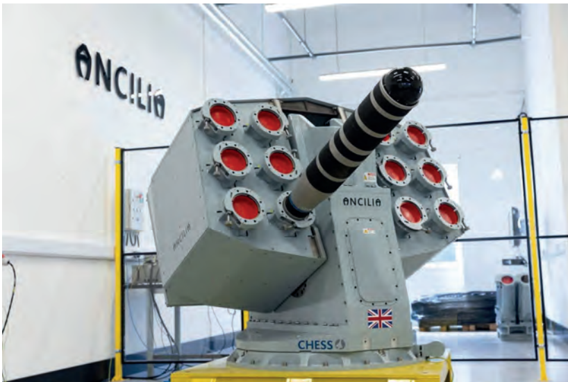
ANCILIA IS SMALL, LIGHTWEIGHT, CAPABLE OF FIRING MULTIPLE COUNTERMEASURES, AND CAN SWIVEL RAPIDLY AND ADJUST THE ANGLE DECOYS ARE FIRED AT
