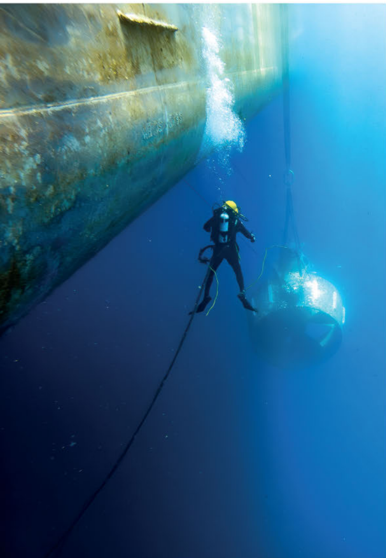
AN OFFSHORE VESSEL THRUSTER ON ITS WAY UP FOR OVERHAULING, UNDER THE SUPERVISION OF AN SGS DIVER-TECHNICIAN
