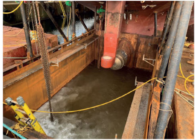
THE REPAIRED RUDDER HORN WITH NEW SHAFT INSTALLED
