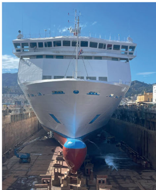
THE MOBY LINES FERRY VINCENZO FLORIO WAS RECENTLY DOCKED AT PALUMBO MESSINA YARD FOR A PACKAGE OF WORK THAT INCLUDED HYDRO BLASTING IN PREPARATION FOR A SILICONE PAINT JOB
