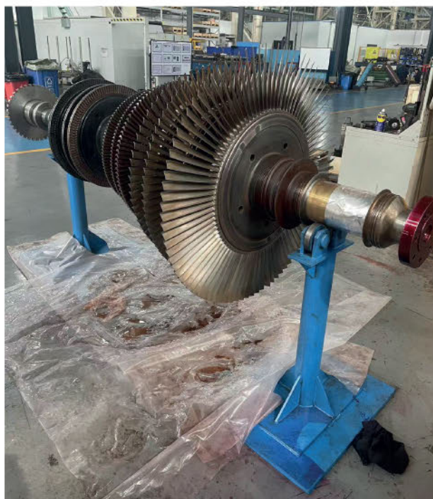
FOLLOWING REVERSE ENGINEERING, SULZER MANUFACTURED NEW BLADES AND REPLACED THE TURBINE, EXTENDING SERVICE LIFE BY UP TO 15 YEARS
