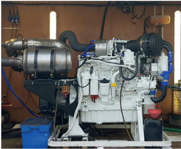
An M&H test engine, running on C14-C16: the company's engines range from 55-667kW (image: M&H Engines)
