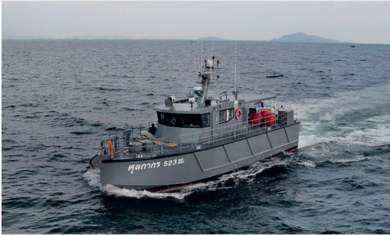
The 20.5m Customs Boat 523 has a cruising range of 300nm
