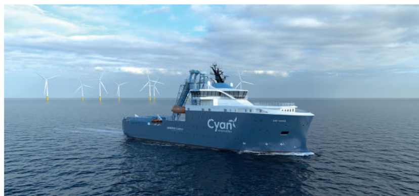
Cyan Renewables' forthcoming SOV will be based on the Vard 4 19 class, modified for a diesel-electric powertrain
