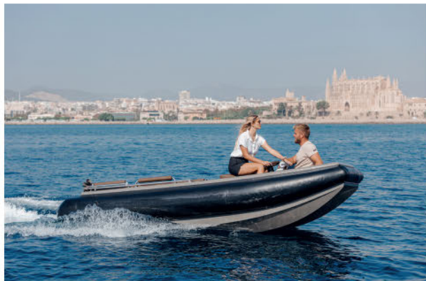
The Ribcat can inflate/deflate its air tube within 45 seconds
