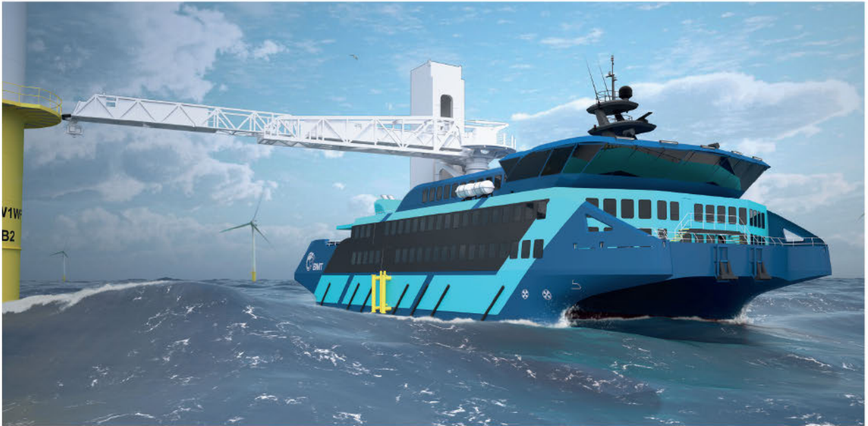
BMT's 'mini-sized', methanol-ready 48m SOV design has been developed to meet current and future energy requirements
