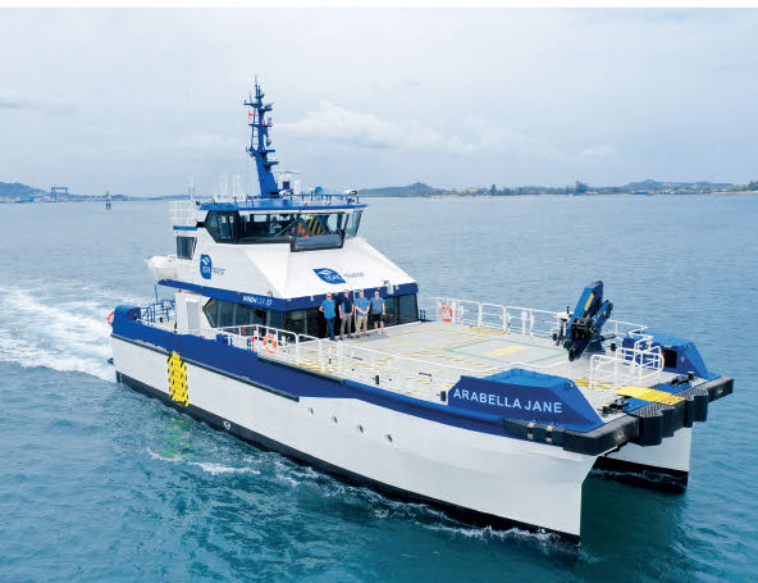
The 27m Arabella Jane , built by Penguin in Singapore, is intended as the last ever diesel-powered CTV to join Tidal Transit's fleet
