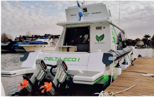
Each of the new electric boats will be powered by twin Torqeedo 12.0 motors and Power 48-5000 batteries
