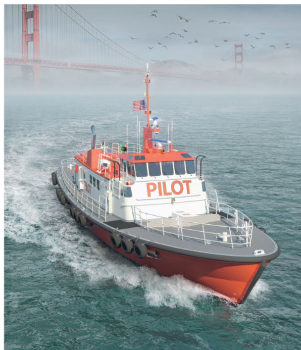
Glosten's new pilot boat design for the SFBP has extended the length by 1.8m, creating room for the installation of batteries (image: Glosten)
