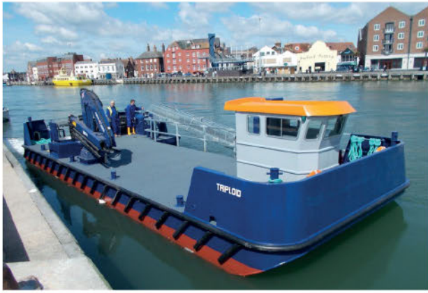
The 15.3m x 6m oyster-harvesting boat Triploid , delivered in 2016, was tailored for the shallow 2m depths of the oyster beds in Poole Harbour, UK
