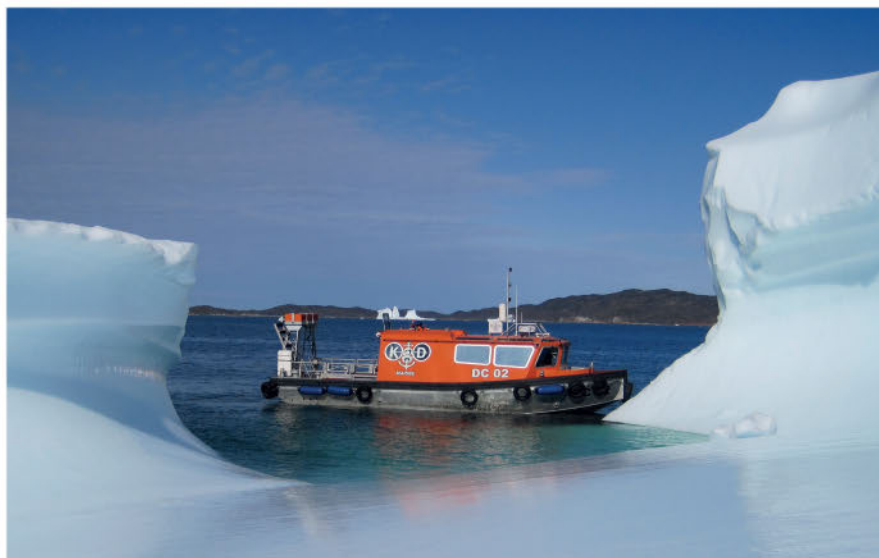
DC01 and DC02 (pictured) were constructed as subsea intervention daughter craft for KD Marine, initially for operations around North Sea offshore platforms: the 11.9m x 3.6m sisters were delivered in 2010
